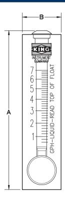
Economical machined cast acrylic block construction makes these meters great for OEM use. Optional inlet metering valve available
